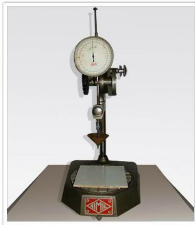
**Fig. 31.1 Cone Penetrometer**
